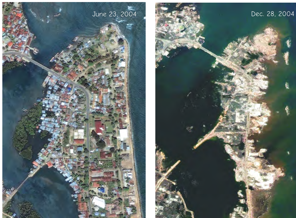
Figure 1-5: GIS may aid in disaster assessment and recovery. These satellite images from Banda Aceh, Indonesia, illustrate tsunami-caused damage to a shoreline community. Emergency response and longer-term rebuilding efforts may be improved by spatial data collection and analysis (courtesy DigitalGlobe).
