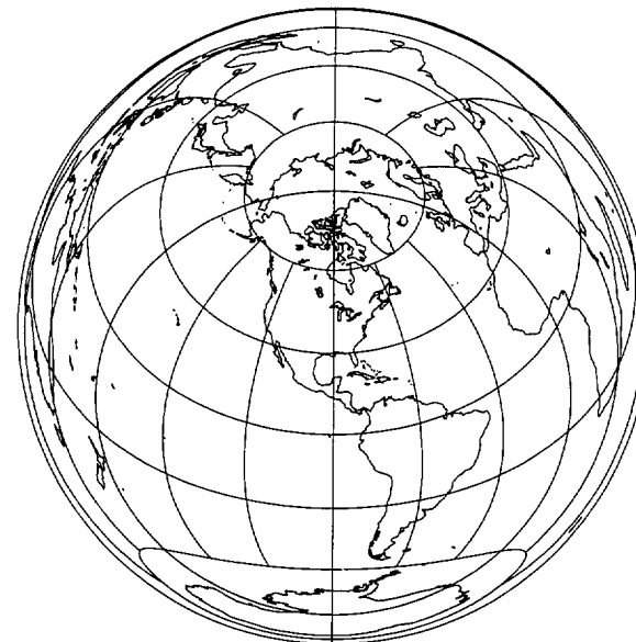
Figure 53E.—Oblique Lambert Azimuthal Equal-Area projection, with shorelines, 30° graticule, central latitude 40° N. Central meridian 90° W. Range 180° (world map).
