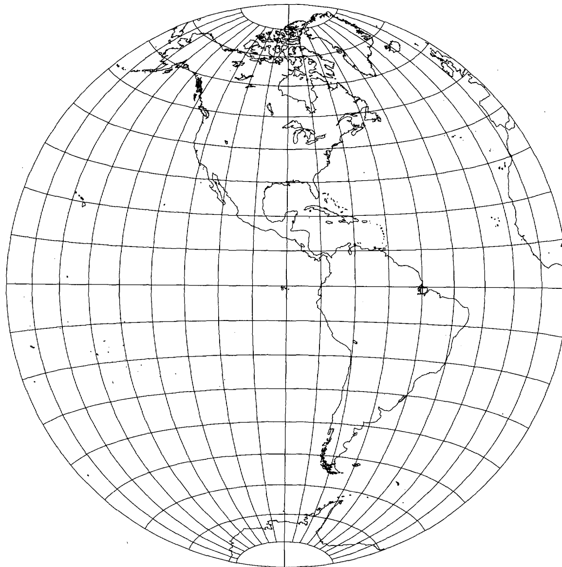
Figure 53C.—Equatorial Lambert Azimuthal Equal-Area projection, with shorelines, 10° graticule. Central meridian 90° W. Range 90°.
