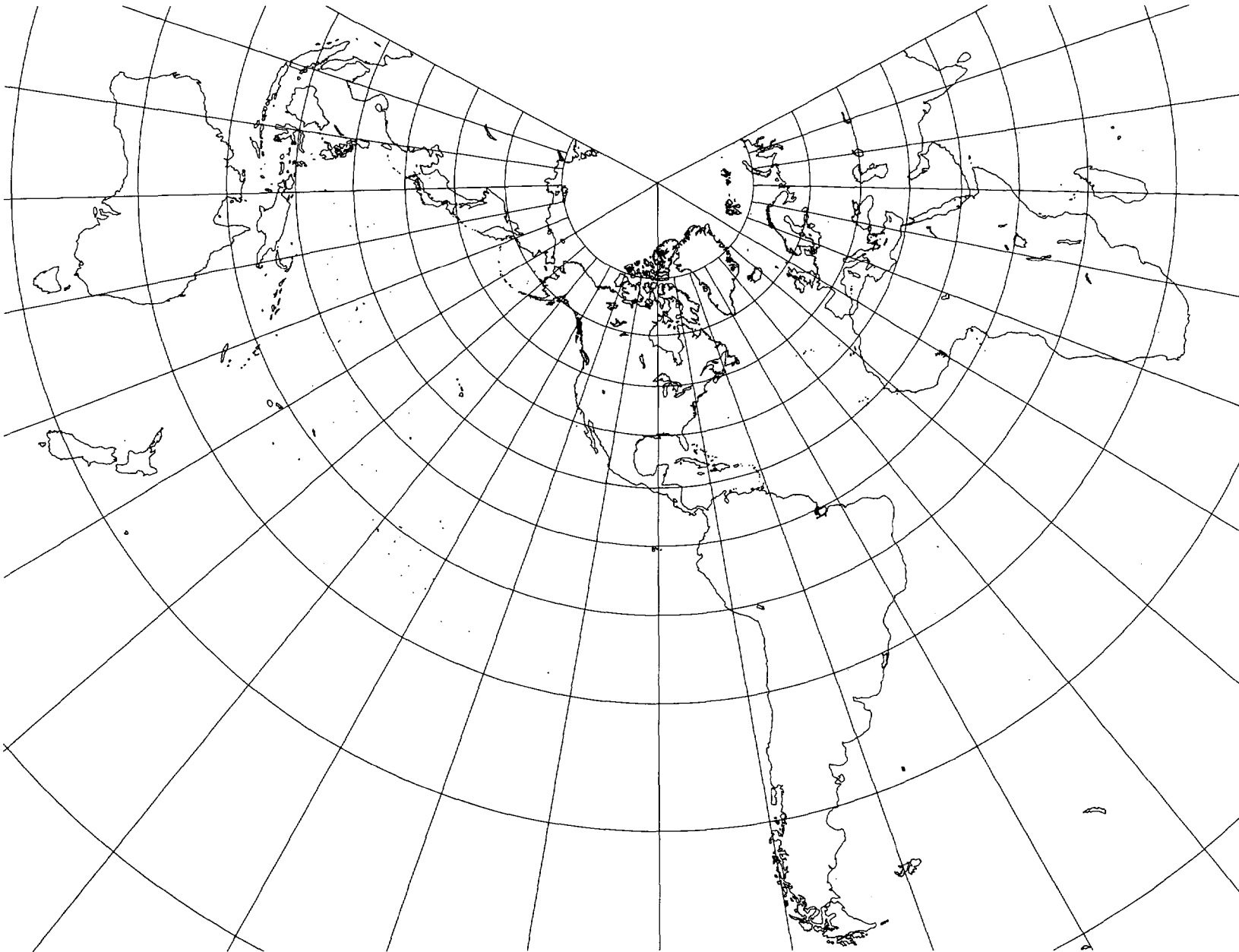
Figure 38B.—Lambert Conformal Conic projection, with shorelines, 15° graticule. Central meridian 90° W. Standard parallels: 20° and 60° N.
