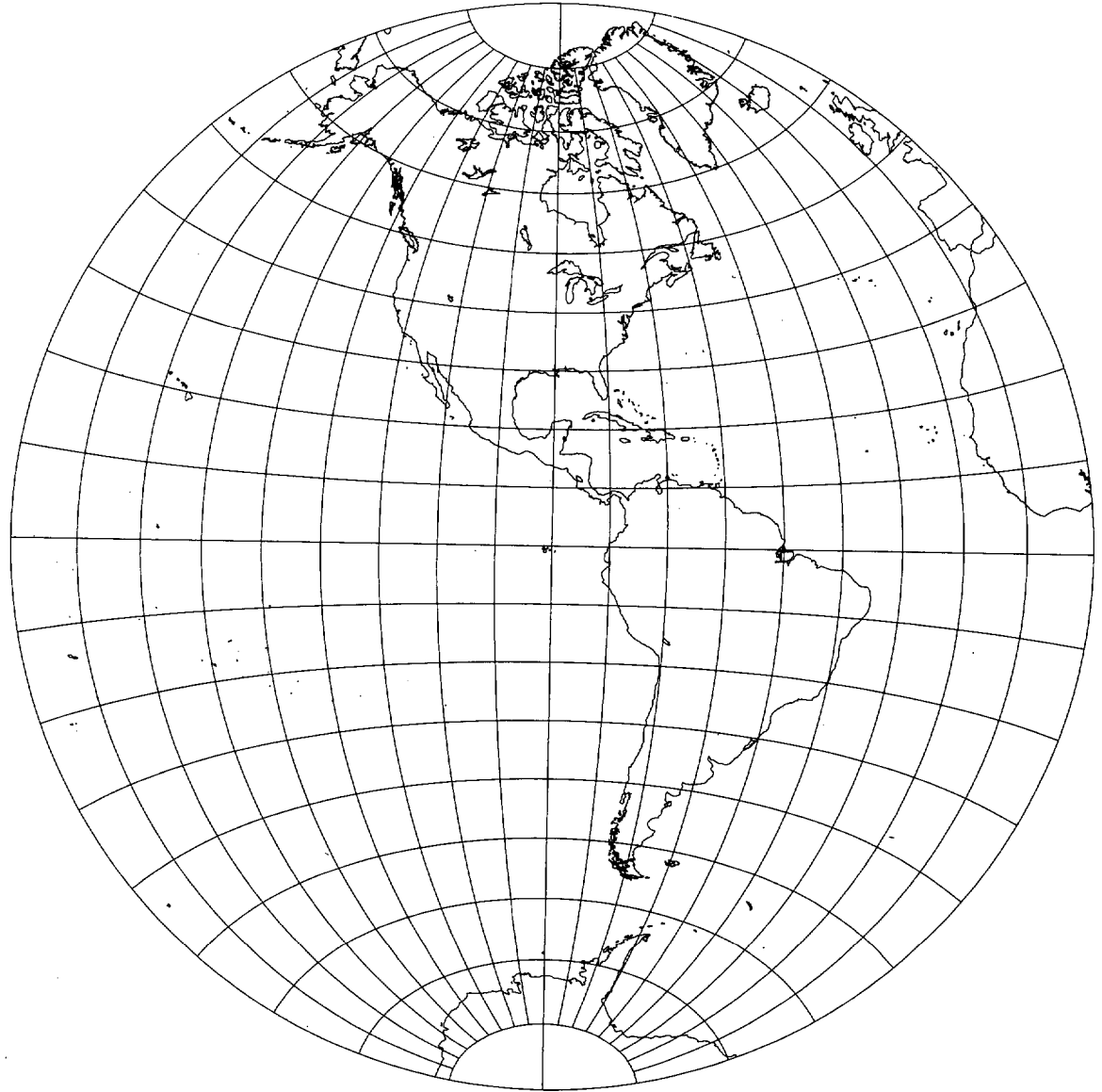
Figure 54C.—Equatorial Airy projection, with shorelines, 10° graticule. Central meridian 90° W. Range 90°.
